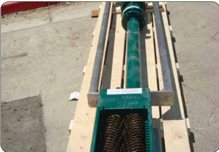
Muffin Monster with lifting bail (*optional extended shaft)
