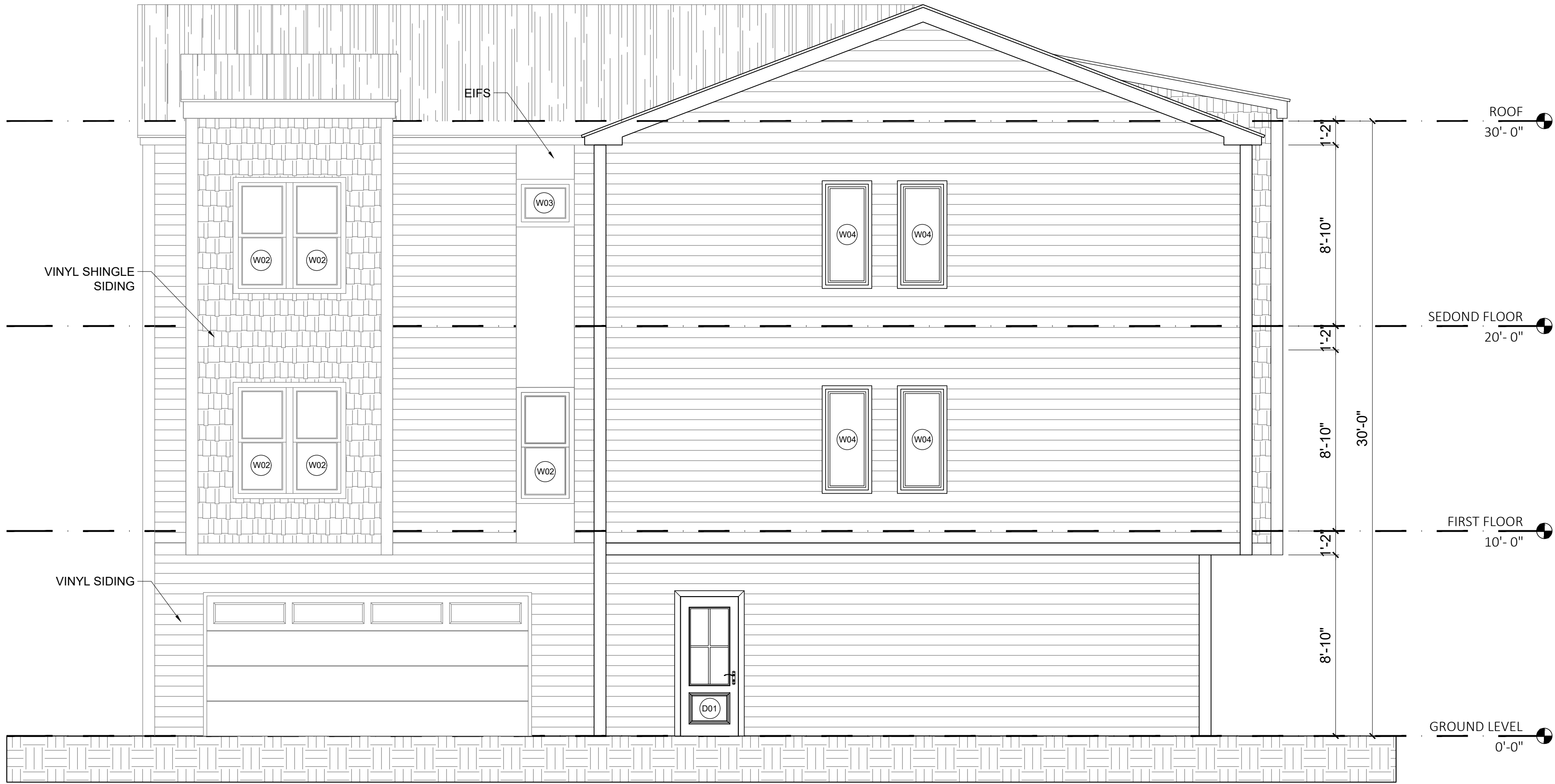
7 UNITS 1, 2, 3, 4 SIDE ELEVATION 1/4" = 1'-0"
