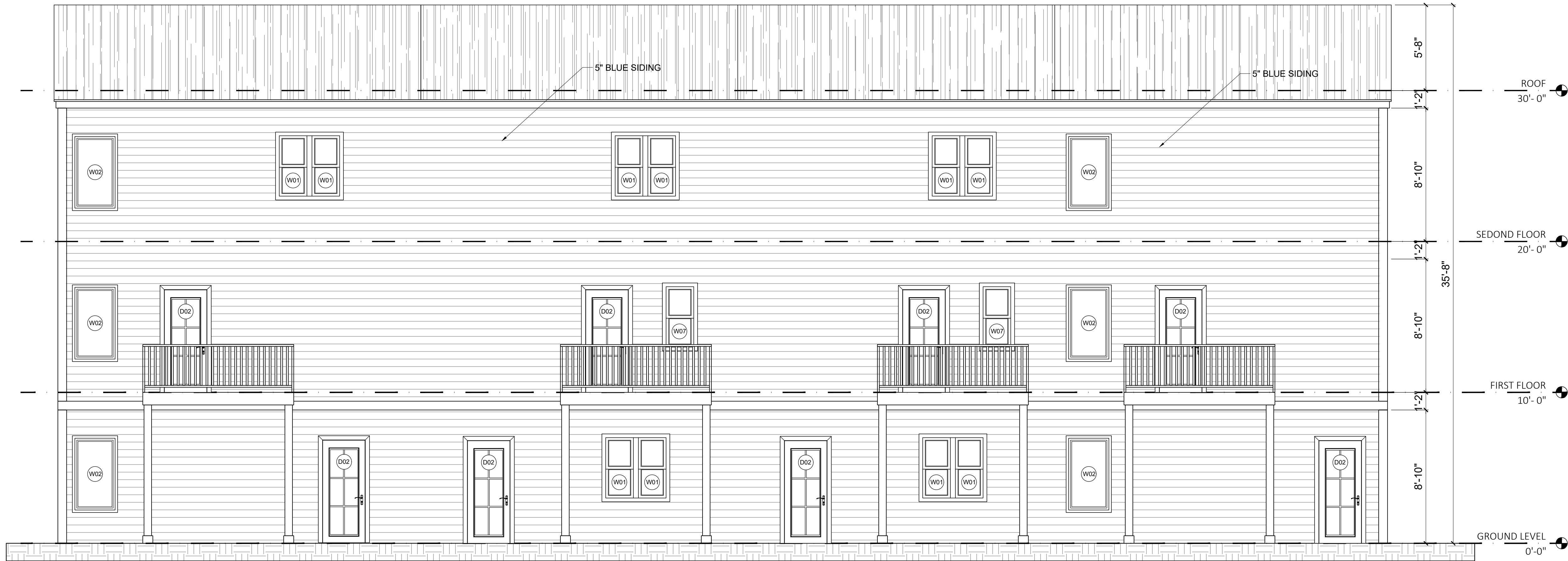
8 4-UNIT NORTH ELEVATION 1/4" = 1'-0"
