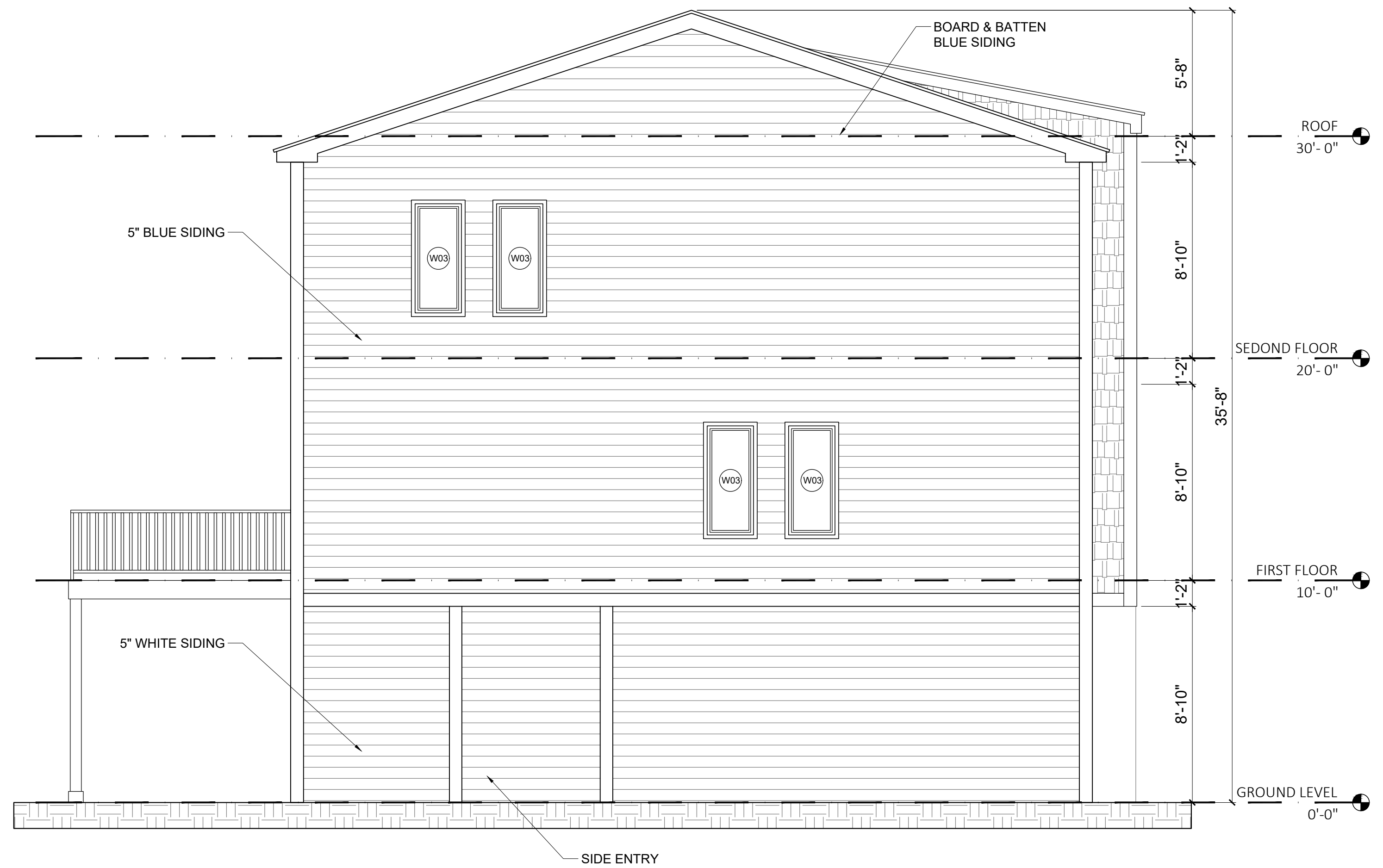
10 4-UNIT WEST ELEVATION 1/4" = 1'-0"
