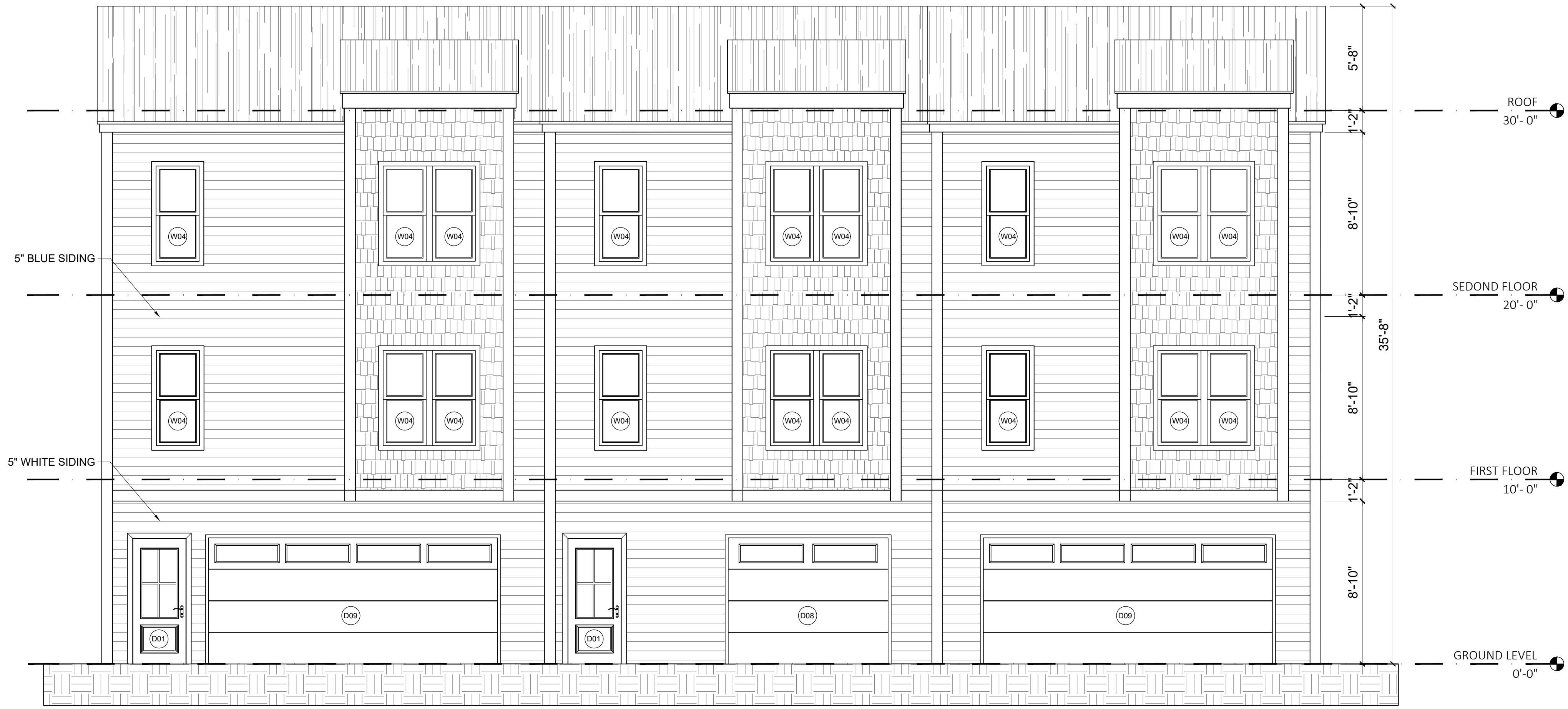
16 3-UNIT WEST ELEVATION 1/4" = 1'-0"
