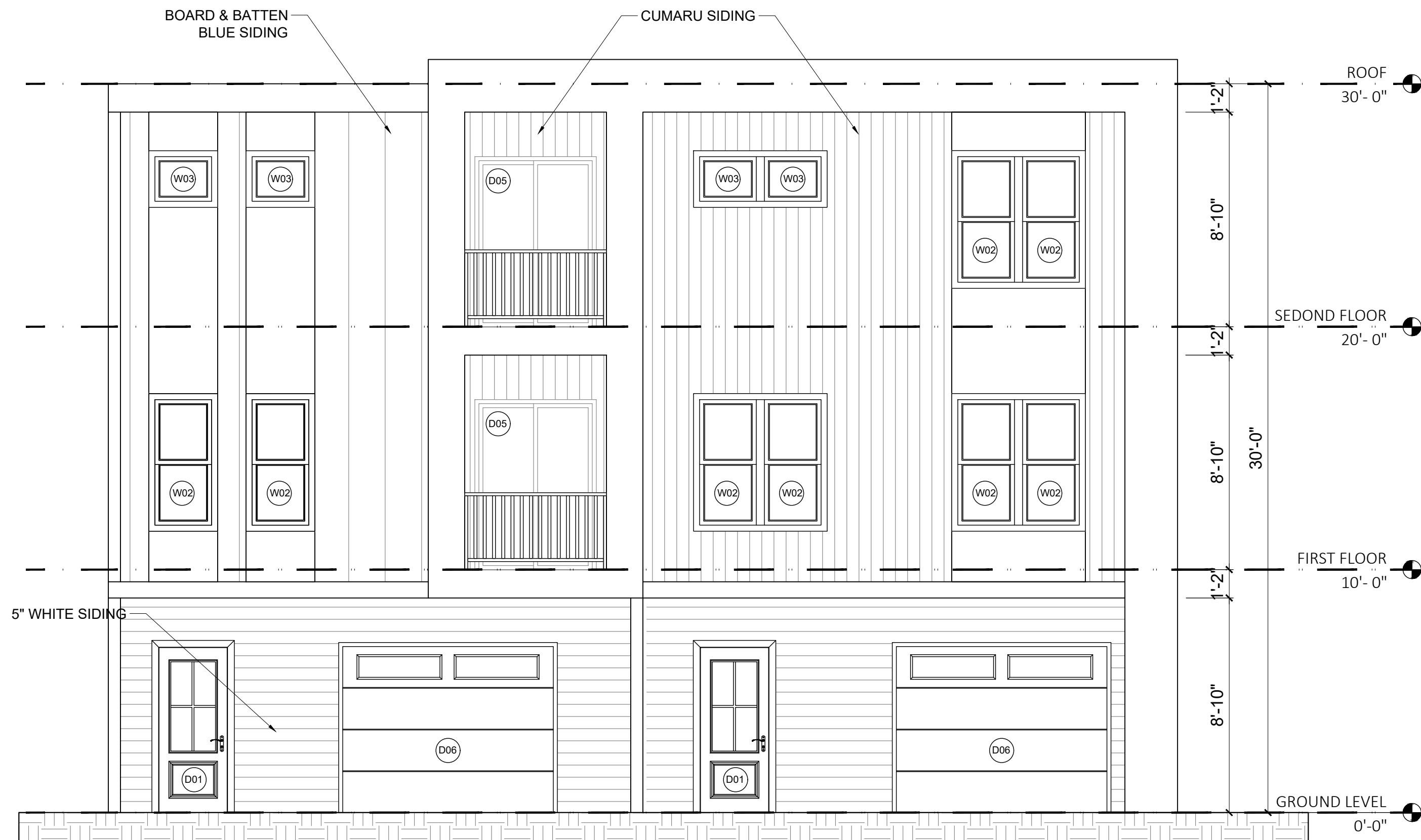
15 UNITS 4 & 5 FRONT ELEVATION 1/4" = 1'-0"
